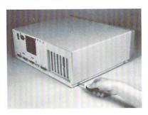
Remove the center screw from the rear of the Amiga. Be careful to unscrew the correct screw as shown.
