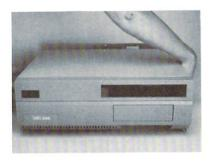
If the cover gets stuck, do not force it. Look under the top of the cover towards the middle. Check to see if any wires or cables are caught under the small projection where the middle screw had been attached. If anything is caught, gently untangle it, and continue to slide the cover off.
